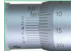
Spindel 0,5 mm - Ablesung 0,001 mm Thread pitch 0.5 mm - Reading 0.001 mm
