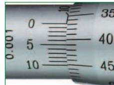
Spindel 0,5 mm - Ablesung 0,001 mm Thread pitch 0.5 mm - Reading 0.001 mm
