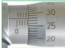
Spindel 0,5 mm - Ablesung 0,01 mm Thread pitch 0.5 mm - Reading 0.01 mm
